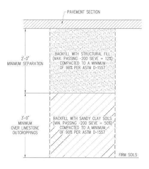
EXCAVATE AND BACKFILL DETAIL
